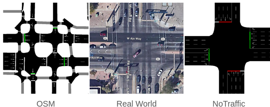
Figure 3: Intersection layout: OSM, Real-World, NoTraffic™ generated intersection.
