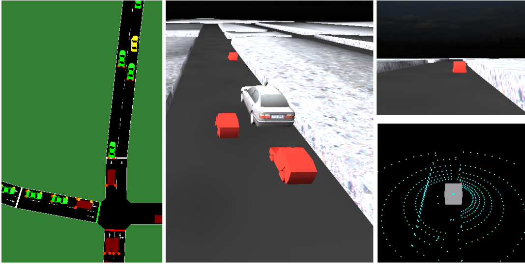
Figure 7.3: Validation of second functionality test. On the first row, SUMO view is presented followed by USARSim. The camera and LIDAR sensor from the reflective agent is depicted in last.
