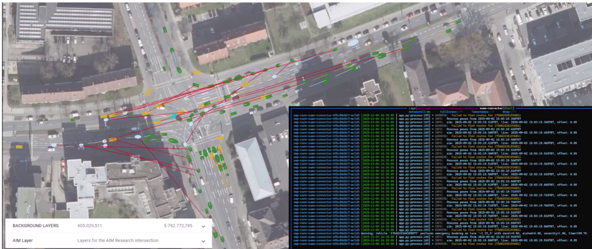
Figure 5. Snapshot of the dashboard for live traffic visualization (background map: GeoBasis-DE/LGLN (2024) CC-BY/4.0).
