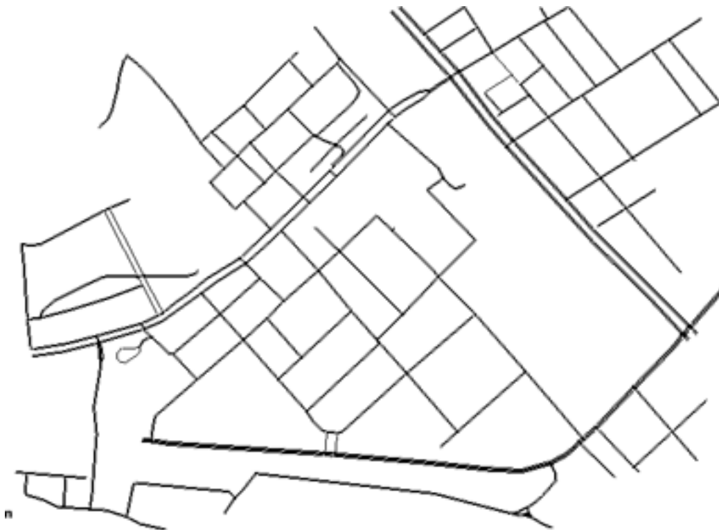
Figure 5.2. A network where the usage of random routes causes an improper behaviour due to the mixture of rural and minor roads
