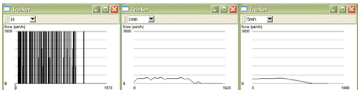
Figure 7.4. A sample usage of the aggregation option (for an induction loop in this case, for aggregation times of 1s, 1min, 5min (from left to right))
